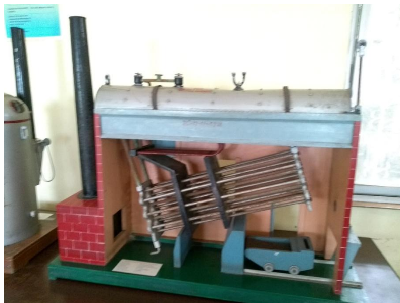
CUT MODEL OF BABCOX & WILLCOX BOILER
