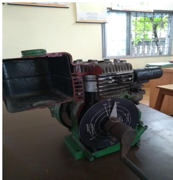
CUT MODEL OF 4S PETROL ENGINE
