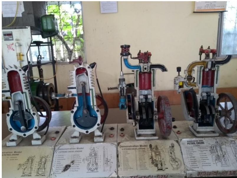
CUT MPDEL OF 4S & 2S DIESEL AND PETROL ENGINE
