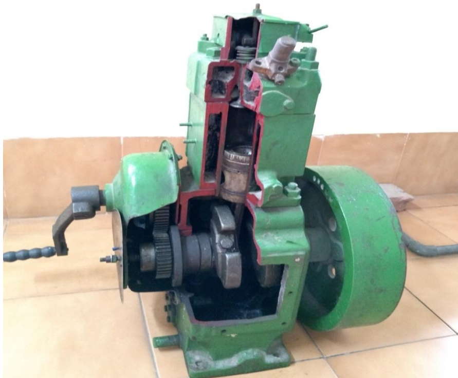
CUT MODEL OF 4S DIESEL ENGINE
